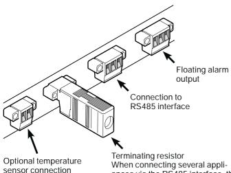
When connecting several appliances via the RS485 interface, the terminating resistor must remain on the last appliance. Remove the terminating resistors from the appliances in
